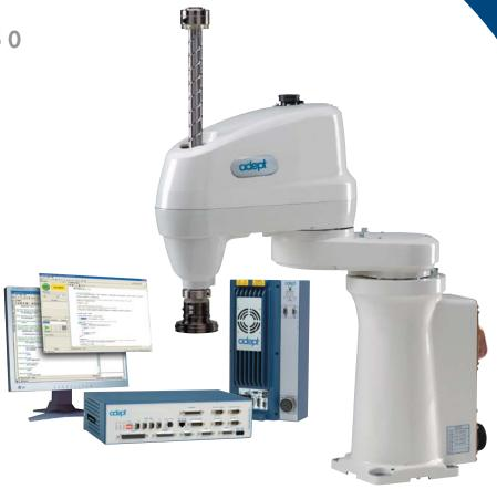
The Adept Cobra s350 features a small motion envelope while maintaining high speeds and payloads. It can be used in mechanical assembly, material handling, packaging, machine tending, screwdriving, and many other operations requiring fast and precise automation. The Adept Cobra s350 series robot has a 350 mm reach.
