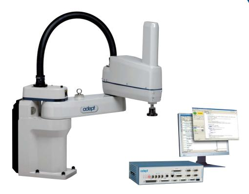
The Adept Cobra s600 is an affordable, high-performance robot system for mechanical assembly, material handling, packaging, machine tending, screw driving, and many other operations requiring fast and precise automation.
