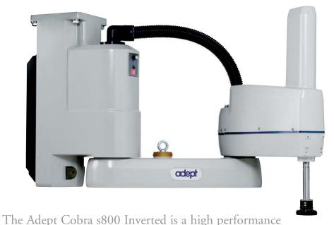
robot system designed for packaging and material handling applications. The overhead mounting makes it ideal for mounting above a conveyor belt and minimizing the machine footprint. With an 800 mm reach and 5.5 kg payload this robot is well suited for a wide range of applications.
