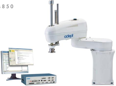
The Adept Cobra s850 4-degrees of freedom Scara robot is a highperformance robot system for case and carton loading, mechanical assembly, material handling, packaging, machine tending, screwdriving, and many other operations requiring fast and precise automation. Adept Cobra s850 robots are available in standard, inverted and IP65 configurations that offers the highest flexibility.
