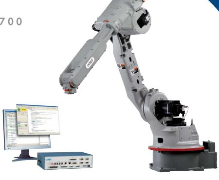
The Adept Viper 6-axis robot family is a high-performance line of robots designed for a wide variety of applications. The speed and precision of the Adept Viper robots make them ideal for assembly, material handling, packaging, machine tending and many other operations and applications that require fast and precise automation. The Adept Viper s1700 six-axis robot is an extended-reach and higher payload robot that complement the Viper product family.
