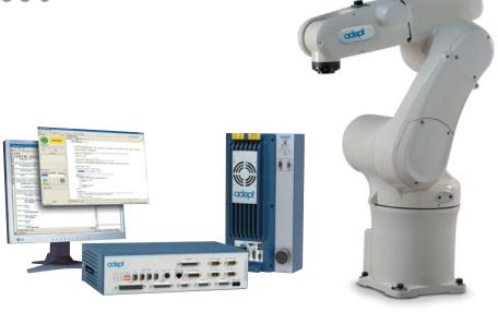
The Adept Viper 6-axis robot family is a high-performance line of robots designed specifically for a multitude of applications. The speed and precision of the Adept Viper robots make them ideal for assembly, material handling, packaging, machine tending, medical, pharmaceutical and many other operations requiring fast and precise automation. The Adept Viper product family is available in standard, clean-room and IP65 versions for both the Adept Viper s650 and Adept Viper s850 robots.
