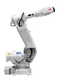
The IRB 6640 is available in different arm lengths and matching handling capacities. It is based on proven components from earlier generations, to ensure ease of maintenance and exchangeability as well as high up time.
